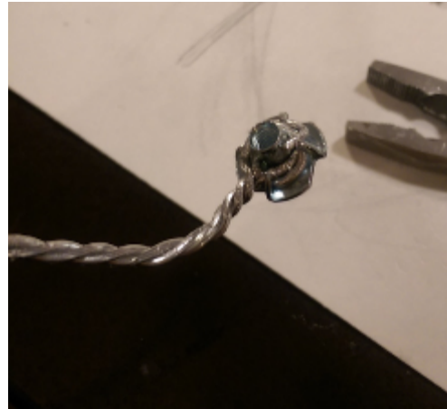
For the feet the legs are bent 90 degrees to the front and a nut is attached to them, so the puppet can be bolted to a surface to make a walking or dancing effect. In this case I attached t-nuts for the flying woman and a normal nut for the dancer (because she needed to appear to be on point).
