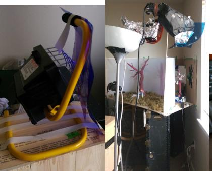
In the front of the cyclorama there was one incandescent side light on the left with first a green and then a purple gel; on the right side, I used two incandescent lights on a dimmer: one with a blue gel and the other with a dark yellow gel. I clamped these two lights on a standing lamp that I used as a boom.
